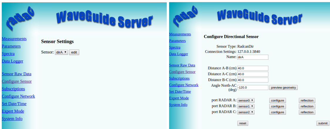
Figure 3.2: The "configure sensor" page will display a sensor drop-down menu. Choose "dirA" and click "edit". This will display the configuration page for the WaveGuide Direction radar sensors.
