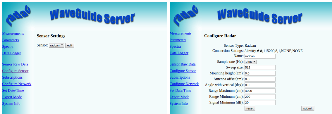
Figure 3.3: The "configure sensor" page will display a sensor drop-down menu. Choose "radcan" and click "edit", this will display the configuration page for the radar sensor.
