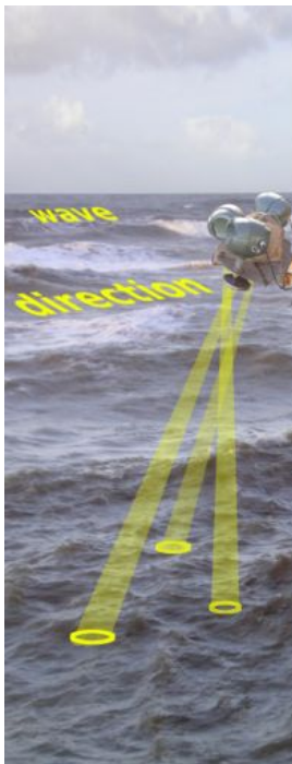
Figure 3: Radar A looking perpendicular downward. Radars B and C tilted by 15^\circ [deg].
